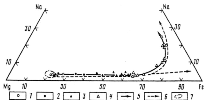
Fig. 1. Compositional variations of clinopyroxenes from alkalic lavas of the Central Range, Kamchatka, in the system Mg-Fe-Na: 1 to 4) points for clinopyroxenes from 1) alkalic olivine basalt, 2) trachyte and 3, 4) trachyrhyolite and comendite [3] crystal cores, 4) outer zones]; 5, 6) crystallization trends of clinopyroxenes from 5) alkalic lavas, Central Range, Kamchatka, and 6) trachyte and quartz trachyte, Dogo Island, western Japan [5]; 7) field of clinopyroxenes from trachybasalt, Dogo Island [5].
